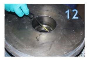
**12.** Clean and inspect stuffing box bore ensure no excessive wear or damage to bore and drive pin (Picture 12). Replace stuffing box if required.
