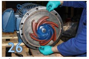
**26.** Install new pump case gasket, and install case and tighten up nuts.
