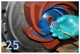
**25**. Install impeller bolt. Note: The bolt is LEFT HAND THREAD.
