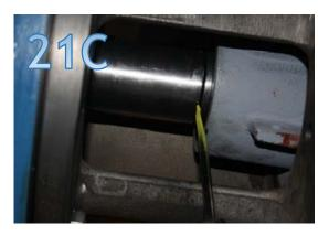
21. Install sleeve with mechanical seal face touching (Picture 21A) and push sleeve onto motor shaft (Picture 21B) until sleeve contacts O-ring.
