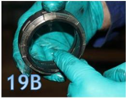
**19.** Apply a thin coat of oil on surface of sleeve and in the bellows of the mechanical seal (picture 19B).
