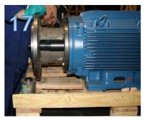
**17**. Install #329 O-ring on motor shaft (Picture 17) up to shoulder.
