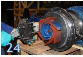
**24.** Using Topco Impeller Wrench (Part #79500) (Picture 24). Thread on (install) impeller in the clockwise direction.
