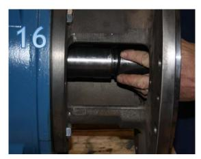
**16.** Install #329 O-ring (Picture 16) on motor shaft up to shoulder.
