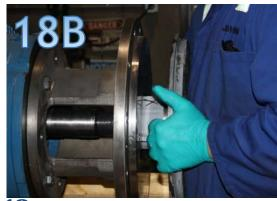
**18.** Install stuffing box onto **C** flange (Picture 18A) to the face (Picture 18B).
