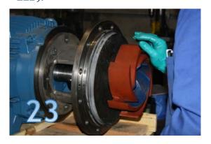
23. Rotate impeller to insure there is no contact with stuffing box (Picture 23).
