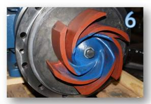
**6.** Using 1 1/8" deep socket, remove LEFT HAND threaded impeller bolt.
