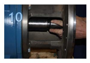
**10.** Remove O-ring (329) from shaft (Picture 10).
