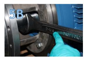
**5.** Secure main shaft on electric motor (Picture 5B) with 2½" open end wrench.
