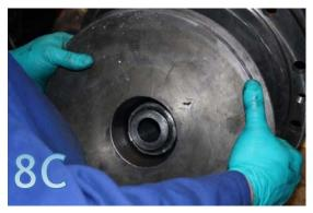
**8.** Remove stuffing box (Picture 8B) from C flange using a <sup>3</sup>/<sub>4</sub>" open end wrench on bolt (Picture 8A).
