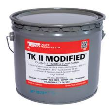
TK II Modified® is a synthetic based thermal compound developed for use in geo-thermal, steam injection and SAG-D projects. This product provides a leak-proof seal in both API and premium connections where elevated temperatures and higher pressures are determining factors. The finely powdered metals prevent over torque, galling, and seizure during connection make-up and break-out. Chemical inhibitors minimize the effects of corrosive environments.
